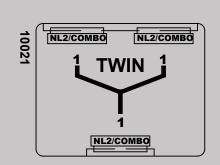
Note the TWIN uses an NL2/Combo connector which can receive a 1/4" connector, an NL2 as well as an NL4 connector (pin1+, pin1- only).
